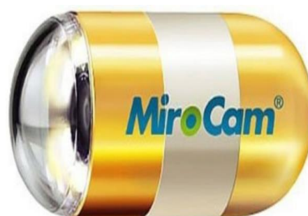
Figure 2. "MicroCam" endoscopic capsule which is used for the examination process.
